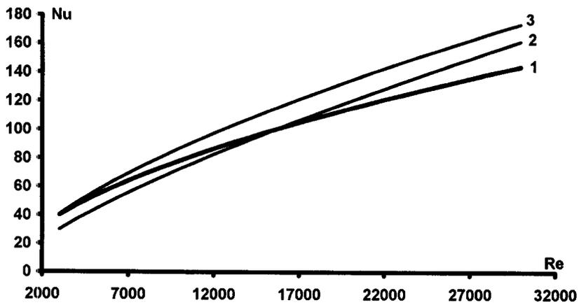
Fig. 7. Mean heat transfer coefficient on a circular cylinder in cross-flows of free stream turbulence intensities of 11–12%: (1) present results (blockage ratio 12%); (2) results in the pilot plant [23] (blockage ratio 17–40%); (3) from Dyban *et al.* [5] (blockage ratio 25%).
