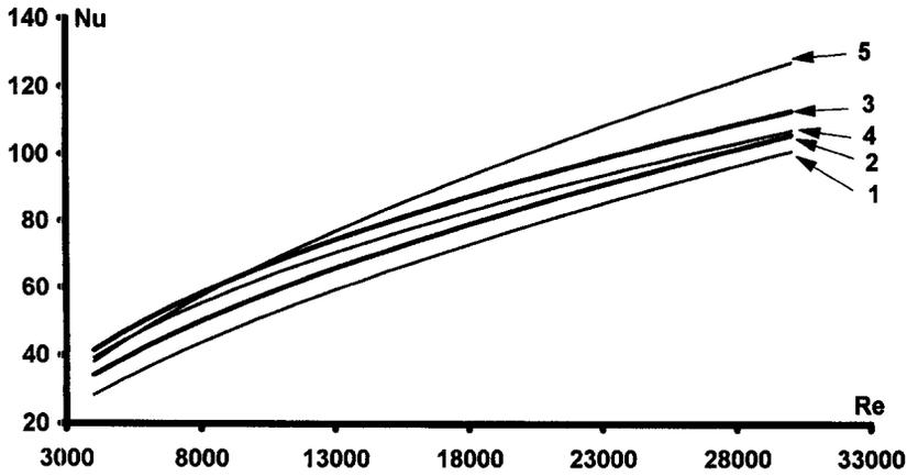
Fig. 6. Mean heat transfer coefficient on a circular cylinder in cross-flows of free stream turbulence intensities close to 0% (1) from Hilpert (quoted by ref. [1]); (2) from Whitaker (quoted by ref. [21]); (3) present results for  $Tu = 1.5\%$ ; (4) extrapolated results for  $Tu = 0\%$ ; (5) from Dyban *et al.* [5].
