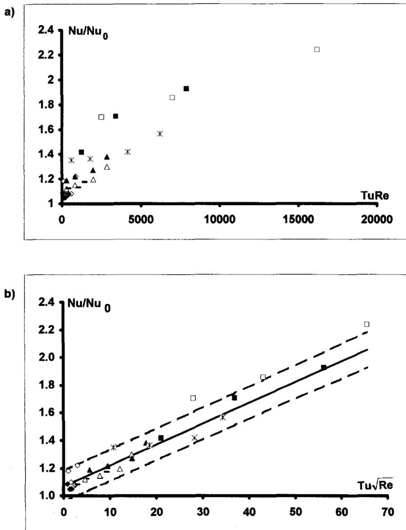
Fig. 10. Transfer intensification:  $Nu/Nu_0$  for the circular and the elliptical cylinders: (a) described using  $Tu Re$ ; (b) described using  $Tu\sqrt{Re}$ . The symbols are the same as in Fig. 11. The dash lines correspond to the calculated 95% confidential limit.
