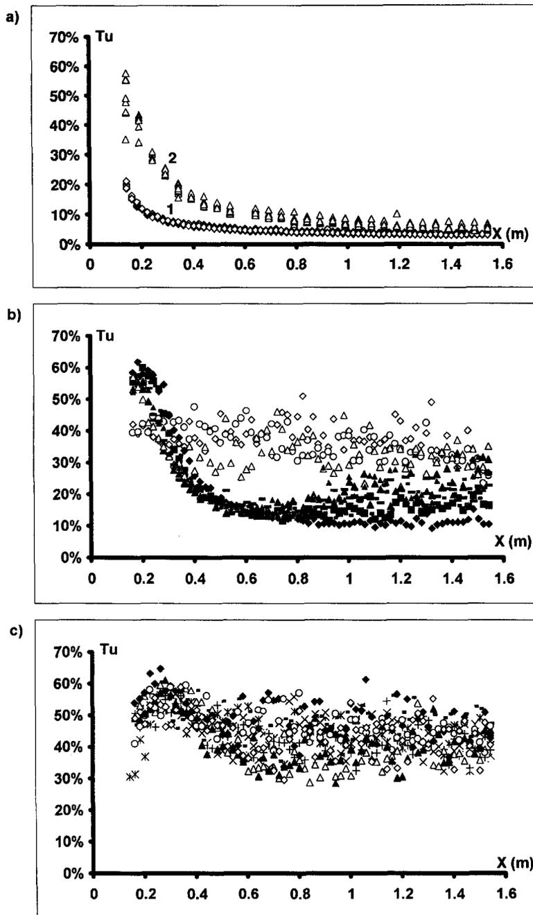
Fig. 4. Free stream turbulence intensity as a function of the distance  $X$  from the perforated plate. (a) (1) plate  $\Phi_g = 18$  mm,  $\sigma_g = 46\%$ ; (2) plate  $\Phi_g = 40$  mm,  $\sigma_g = 46\%$ ; for the sake of clarity the nine points of measurements are represented here by the same symbol. (b)  $\Phi_g = 50$  mm,  $\sigma_g = 33\%$ . (c)  $\Phi_g = 100$  mm,  $\sigma_g = 6\%$ . For (b) and (c) the symbols correspond to the measurements points defined in Fig. 3.
