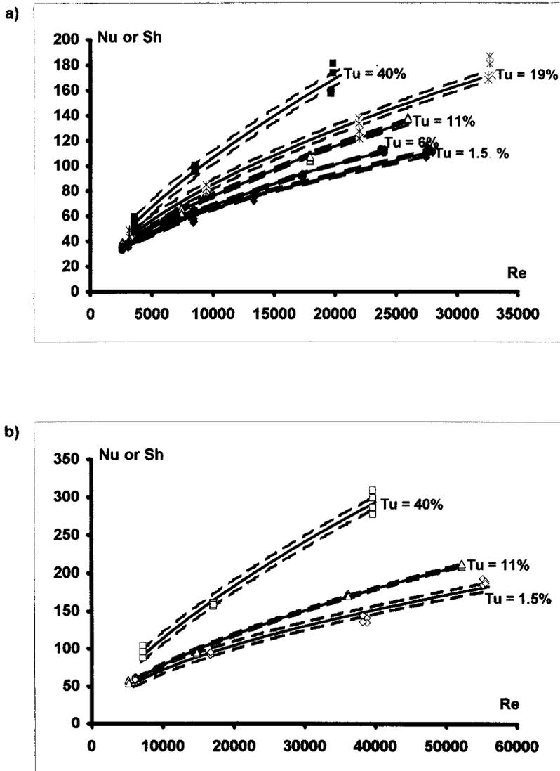
Fig. 5. Values of the transfer coefficients: (a) on the circular cylinder, for free stream turbulence intensities of 1.5, 6, 11, 19 and 40% ( $I_{ref} = d$ ); (b) on the elliptical cylinder  $R = 4$  ( $I_{ref} = a$ ), for free stream turbulence intensities of 1.5, 11 and 40%. The dashed lines correspond to the calculated 95% confidential limit.
