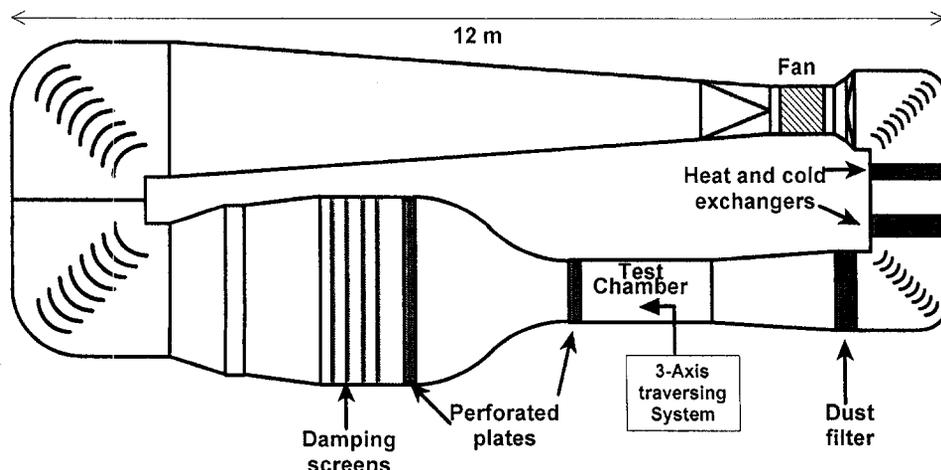
Fig. 2. Schematic representation of the wind tunnel.
