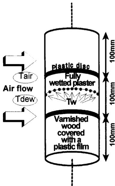
Fig. 1. Diagram of the samples.
