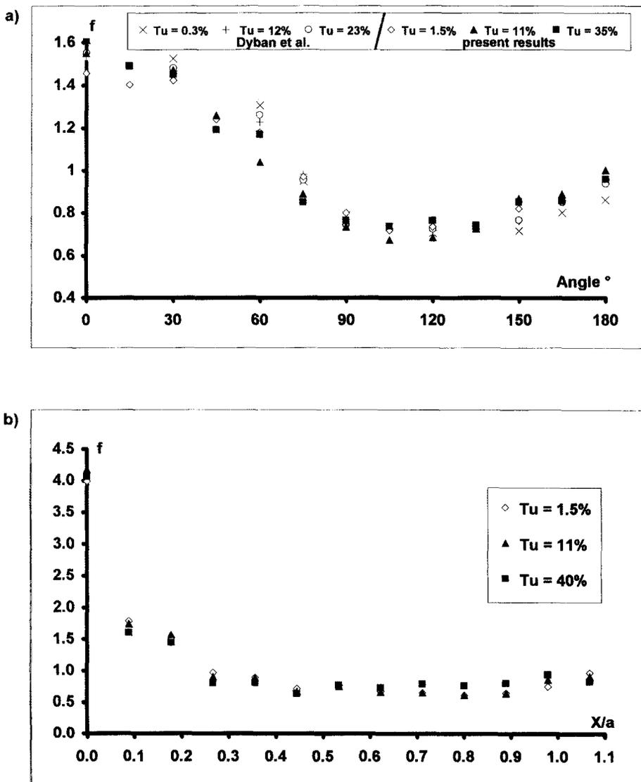
Fig. 9. Evolution of the local transfer coefficients in the form of  $f$  ( $f = h/\bar{h}$ ) along the surface (main stream direction): (a) of the circular cylinder, comparison with Dyban's results for  $Re = 4500$ ; (b) of the elliptical cylinder ( $R = 4$ ); for:  $0.5 \text{ m s}^{-1} < U_\infty < 1.0 \text{ m s}^{-1}$ ,  $1.5\% < Tu_\infty < 40\%$ .
