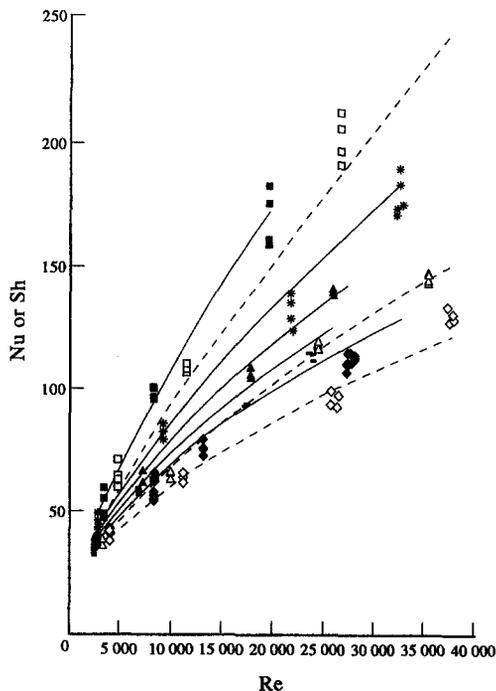
Fig. 11. Experimental mean transfer coefficients on the circular cylinder (solid symbols) and on the elliptical cylinder (open symbols). The calculated values coming from equation (4) are in solid lines and from equation (5) in dashed lines. (1)  $Tu_\infty = 1.5\%$  (diamond); (2)  $Tu_\infty = 6\%$  (dash); (3)  $Tu_\infty = 11\%$  (triangle); (4)  $Tu_\infty = 19\%$  (star); (5)  $Tu_\infty = 40\%$  (square).
