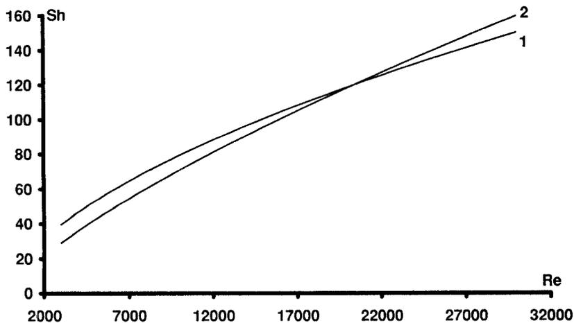
Fig. 8. Mean heat transfer coefficient on an elliptical cylinder ( $R = 4$ ) in cross-flows of free stream turbulence intensities of 11–12%: (1) present results (blockage ratio less than 5%); (2) results in the pilot plant [23] (blockage ratio 5–10%).
