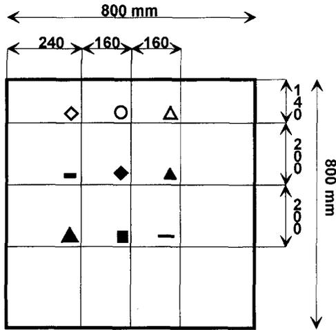
Fig. 3. Localization of the nine points of measurements in a section normal to the flow downstream from a perforated plate.
